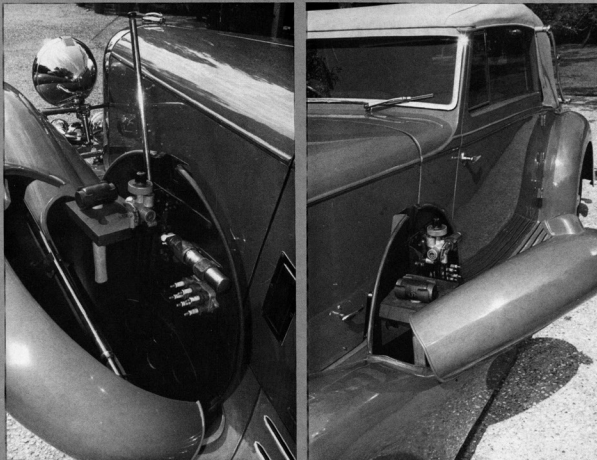
Hydraulic jacking system, tire hammer, spark plugs and auxiliary light nestled in the tire cover of Berta & Jay Leon's 1937 LG45 Drophead Coupe—photos by Ray King
