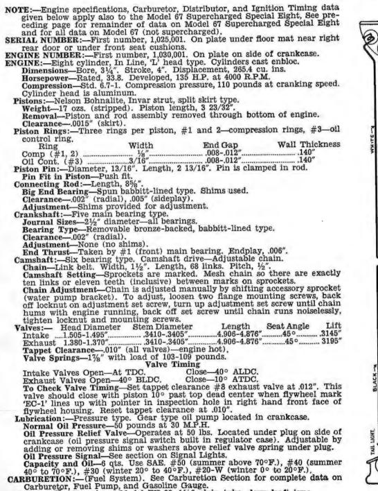
Carburetor, Fuel Pump, and Gasoline Gauge. Carburetor:—Stromberg, Model EX-32, 1½" plain tube, downdraft type. Fuel Pump:—A.C., Type R. Gasoline Gauge:—K-S Telegauge, hydrostatic type.
